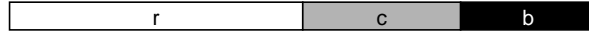
Figure 3: The rcb bank indexing mechanism (cache line interleaving). Hurts the page mode hit rate, but certain memory systems may have justification for using something similar to this.
