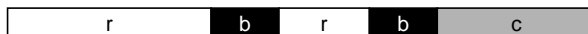
Figure 5: The rbrbc bank indexing mechanism. The best way to index memory banks.
