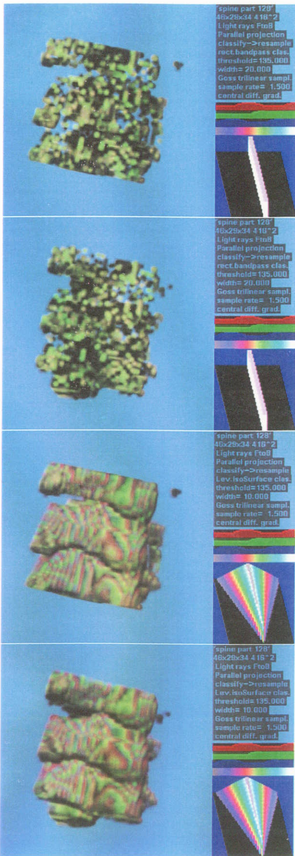
Figure 8: Classifying before resampling creates the same object appearance independent of the viewing angle (here changed by 10 degrees). 6
