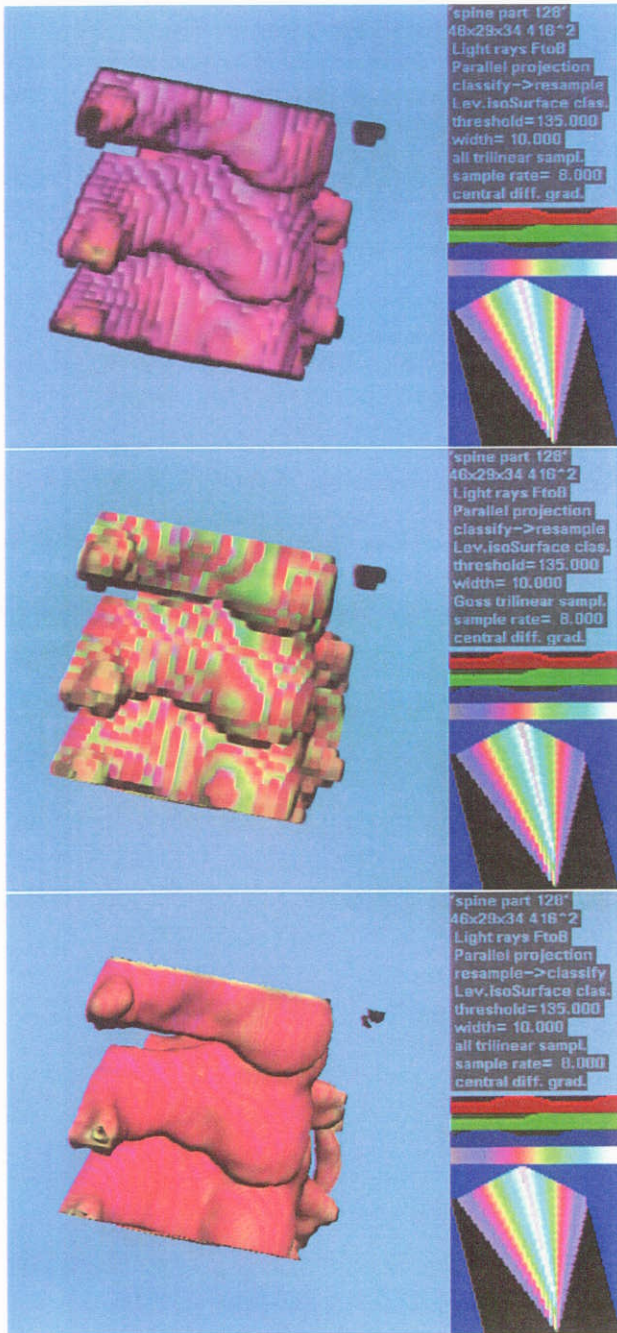
Figure 15: a) Classifying before resampling together with standard trilinear interpolation introduces self occlusion or color shifts. b) Classifying before resampling together with Goss style interpolation is consistent with the reference image c) below. c) Reference image: resampling before classifying together with trilinear interpolation.
