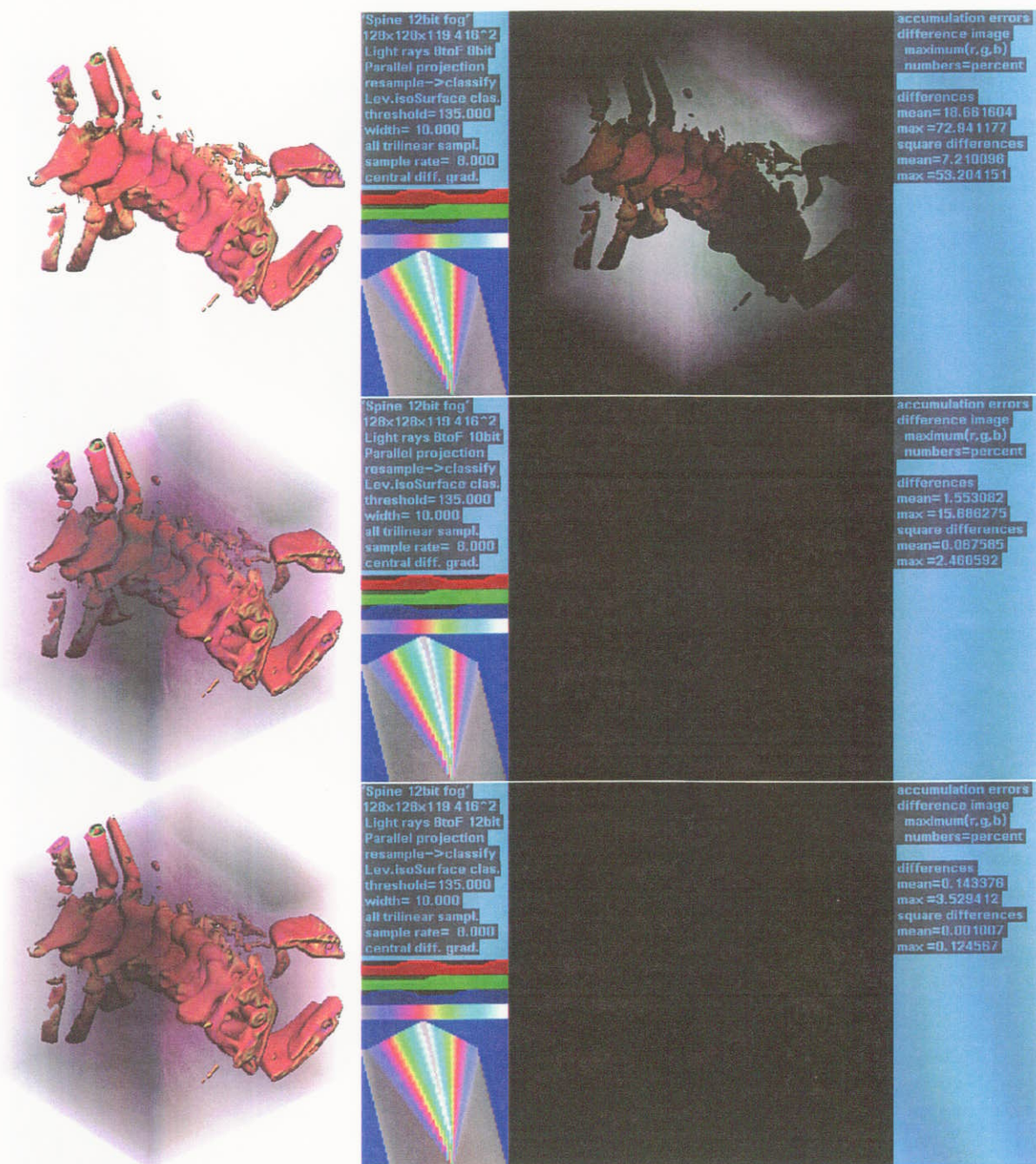
Figure 12: Renderings with limited accumulation buffer sizes 8, 10 and 12 and the difference images towards the double precision accumulation buffer. The images on the left side are rendered using the limited accumulation buffer and the number before the word bits in the third line of parameter informations stands for the number of bits used for that particular image. A zero there stands for double precision. The images on the right side are the difference images of the one left of it and the one using double precision.
