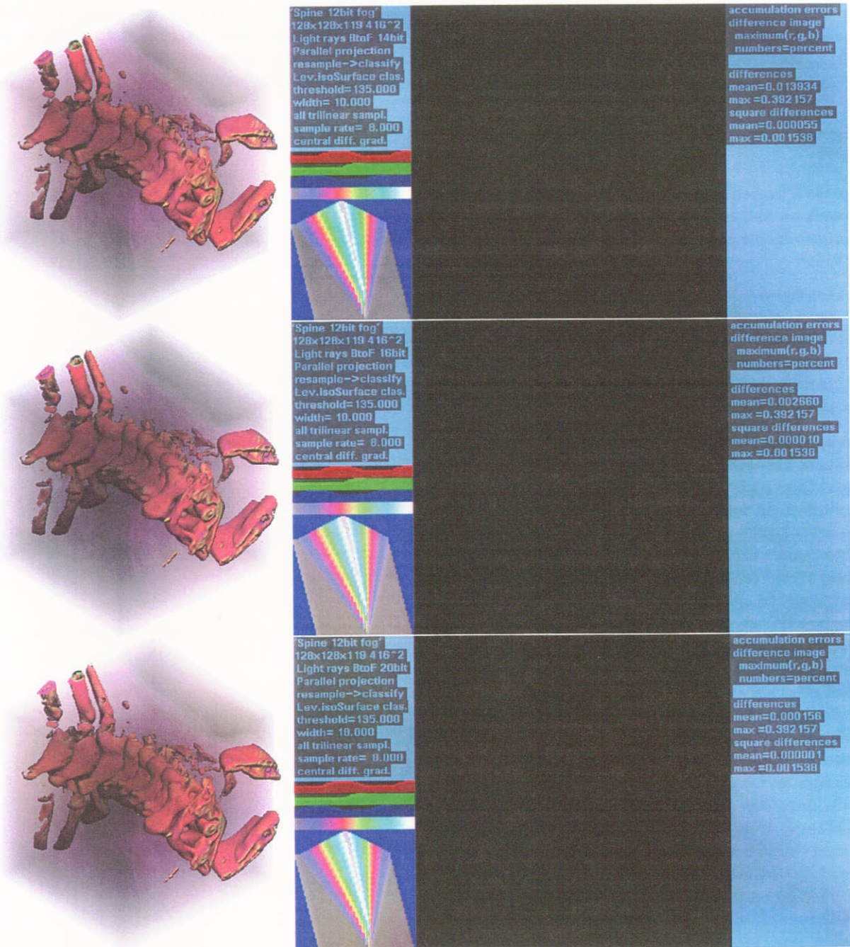
Figure 13: Renderings with limited accumulation buffer sizes 14, 16 and 20 and the difference images towards the double precision accumulation buffer. The images on the left side are rendered using the limited accumulation buffer and the number before the word bits in the third line of parameter informations stands for the number of bits used for that particular image. A zero there stands for double precision. The images on the right side are the difference images of the one left of it and the one using double precision.
