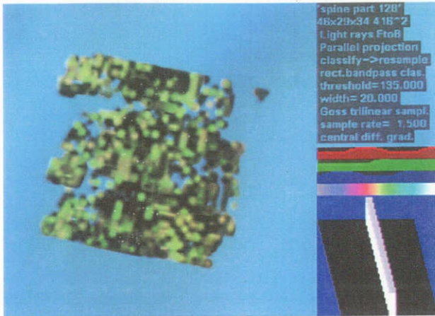
Figure 6: Classifying before resampling together with a very sharp classification function can create a disconnected set of visible voxels.
