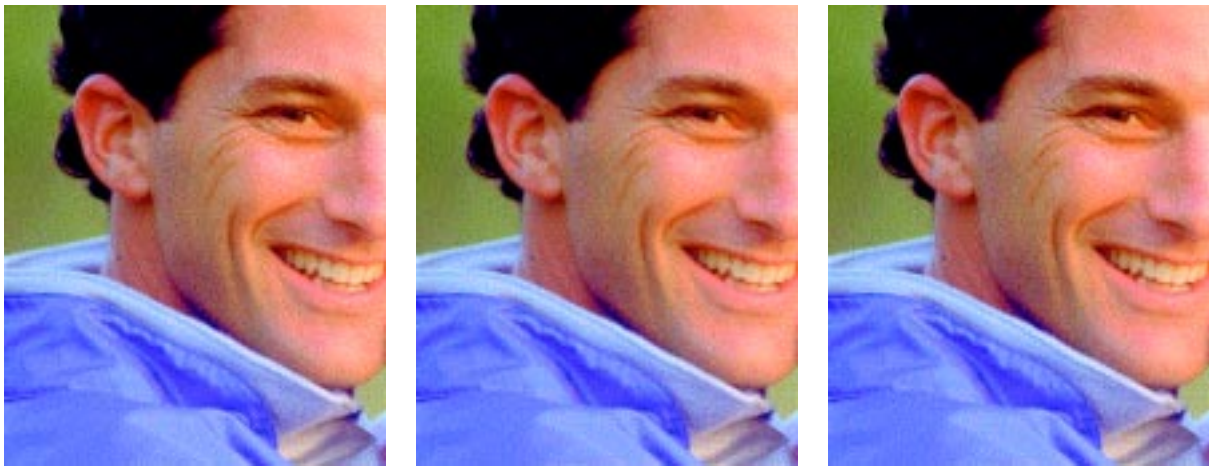
Figure 8: Color corrected results: (a) Error Diffusion, (b) Error Diffusion+Ink Relocation, (c) Ink Relocation disabled on edges.
