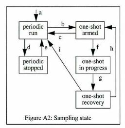
The network state modifications possible from the network via "node-control" are:
