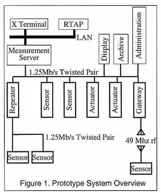
A variety of communication media are used in the demonstration system. An Ethernet LAN is used in the traditional portion of the system. A1.25Mb/s twisted pair and a 49Mhz low-power RF link are used for communication in the distributed portion of the system. A repeater is shown to illustrate the segmentation of the network allowing more nodes than permitted with a single twisted pair. The RF link is built with standard Echelon products.
