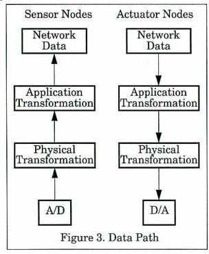
The physical transformation converts between the digital representation in the International System of Units, SI, and the raw digitized representation provided by the transducer. This conversion is based on information from the "electronic data sheet" contained in the transducer.
