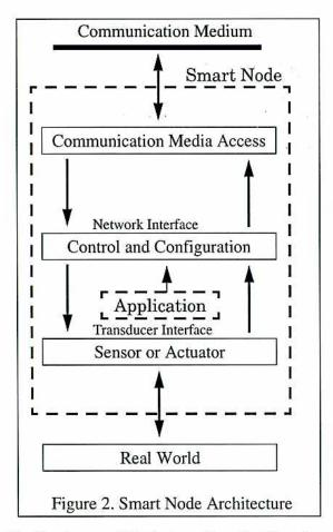
The Communication Media Access block handles the low-level protocol required to
