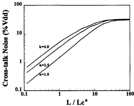
Fig. 8 Cross-talk noise as a function of normalized interconnect length. Cross-talk is improved significantly when  $L < L_c^*$ , but the magnitude of cross-talk is small there.
