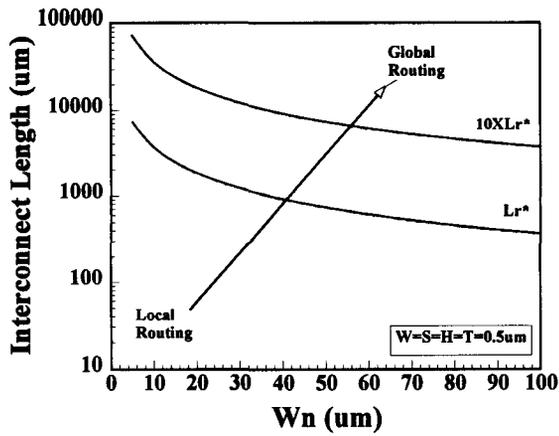
Fig. 6 Critical length  $L_r^*$  for various driver gate width. The plot shows that Cu will not improve the switching time when interconnect length is less than 100um.
