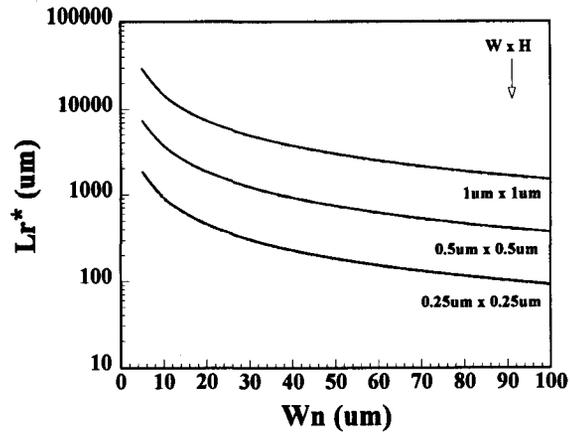
Fig. 7 Critical length  $L_r^*$  for various driver gate width and interconnect metal width and height.  $L_r^*$  is larger than 100um for a (0.25um)x(0.25um) line.
