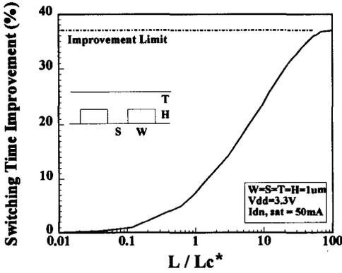
Fig. 2 Switching time improvement with low- $k$  ILD ( $k=2.5$ ) over oxide ( $k=4.0$ ) as a function of normalized length. Switching time is the sum of rise time and fall time.  $L_c^*=84\mu m$ .  $k/k_{oxide} = 37.5\%$  is the improvement limit.
