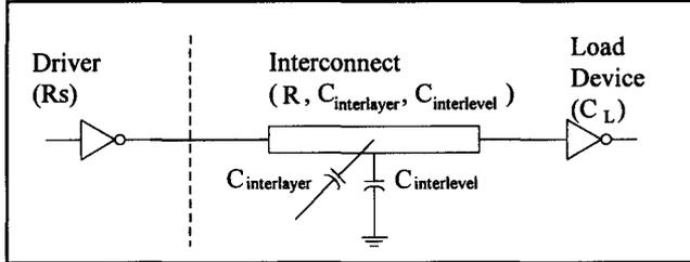
Fig. 1 Schematic of interconnect circuit. Effective source resistance of the driver ( $R_s$ ) is in series with interconnect resistance ( $R$ ), and load device capacitance is in parallel with interconnect capacitance  $C_{interlayer} + C_{interlevel}$ .
