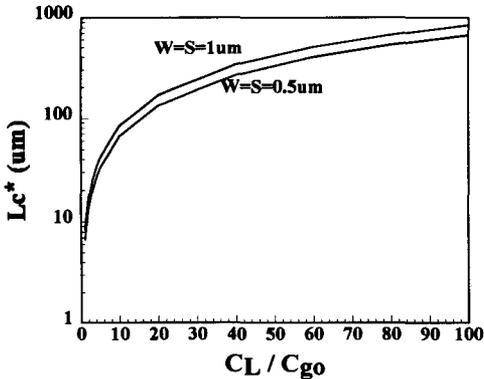
Fig. 4 Critical length  $L_c^*$  for various normalized load device capacitance.  $C_{go}$  is the gate capacitance per micron gate width.
