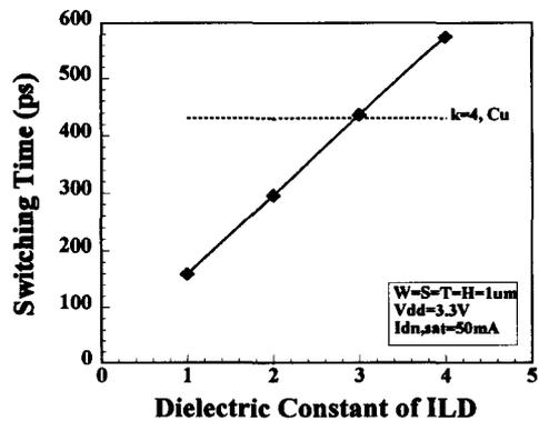
Fig. 5 Switching time as a function of dielectric constant for Al metallization. Switching time of Cu for  $k=4.0$  is also shown for comparison. Interconnect length is  $5\mu m$ .
