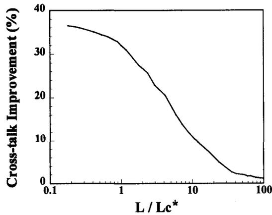
Fig. 9 Cross-talk noise improvement as a function of normalized interconnect length.  $k=2.5$ . No significant improvement is seen when the circuit is interconnect dominated ( $L \gg L_c^*$ ).
