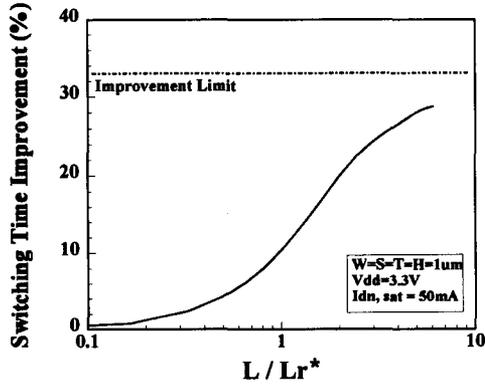
Fig. 3 Switching time improvement with Cu over Al as function of normalized length.  $L_r^*=1500\mu m$ .  $\rho_{Al}/\rho_{Cu} = 33\%$  is the improvement in this numerical simulation.
