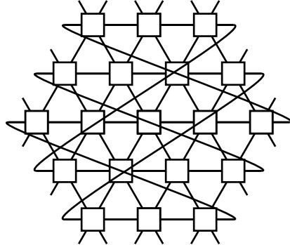
Figure 10: The E3 network. Only one set of wrap links are shown for clarity.
