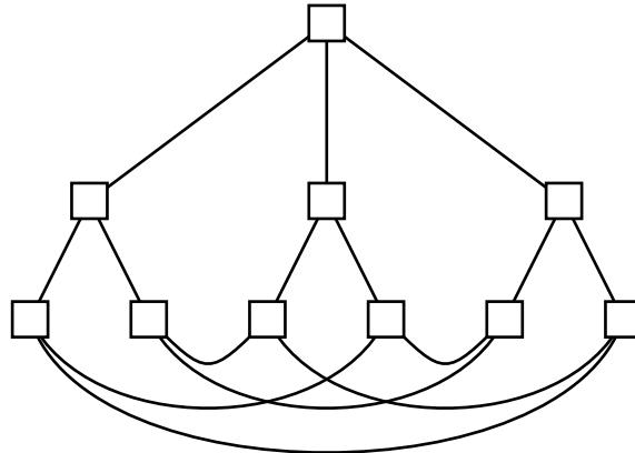
Figure 1: A completely populated spanning tree, with  $b = 3$  and  $p = 2$ , with additional links connecting the leaves.
