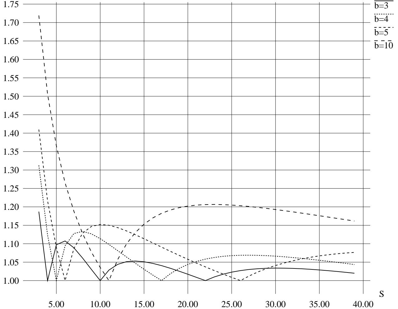
Figure 4: The vertical axis shows the ratio of the spanning tree average path length to the Moore average path length; the horizontal axis is the number of switches, and separate lines are given for branching factors of 3, 4, and 10.
