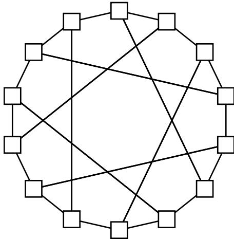
Figure 9: A chordal ring network. This example has fourteen nodes and a chord length of five.
