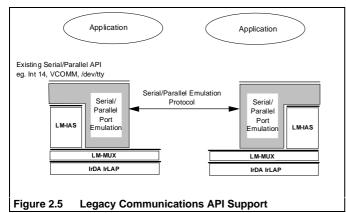
The IrDA has a Working Group known as IrCOM that is working on the emulation of the legacy communication interfaces typically provided by serial/parallel device drivers.
