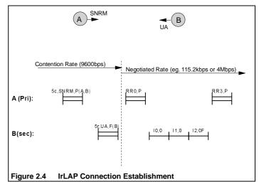
The station addressed by the SNRM responds to the SNRM with an Unnumbered Acknowledge frame, also at the 9600bps contention rate, that contains the results of the negotiation process. At this point both stations apply the newly negotiated parameters. The primary immediately sends an Receiver Ready frame to indicate to the secondary that it is now using the negotiated communication parameters<sup>5</sup>.
