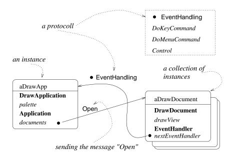
Figure 4: Example Object Diagram
