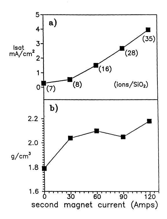
Figure 5. Measurement of a) ion saturation current and b) ECR oxide density as the current is increased in the second magnet of the ECR configuration shown in Figure 2. Ion saturation current is measured with a Langmuir probe and oxide density is measured by RBS. Also shown (in parentheses) is the flux ratio,  $J_f/J_{ox}$ , as a function of the current in the second magnet.
