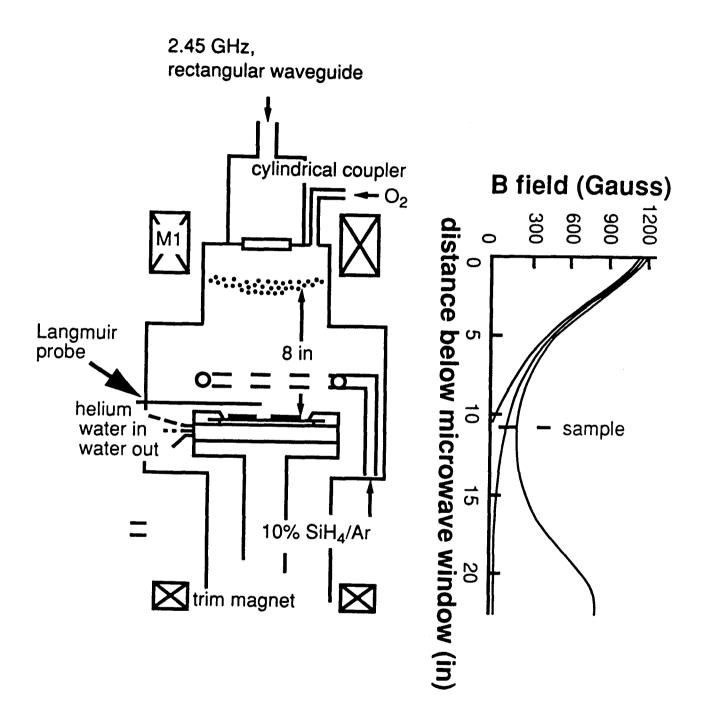
Figure 3. Schematic of ECR PECVD system with a divergent magnetic field source for deposition at high rate. The axial magnetic field corresponding to divergence, collimation and cusp configurations is included.
