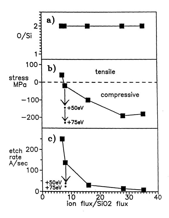
Figure 6. Measurement of a) oxygen-to-silicon ratio, b) oxide stress, and c) wet etch rate as a function of the flux ratio. Oxygen-to-silicon ratio was determined by both Auger and RBS. Stress was measured with a FleXus 2-300i and wet etch rate corresponds to a 10:1  $H_2O$ :HF solution. Also shown are the effects of increasing the mean ion energy to 50 and 75 eV by using rf bias during deposition.
