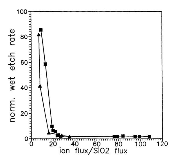
Figure 8. Decrease in wet etch rate in 10:1  $H_2O$ :HF as the flux ratio is increased. Wet etch rate values are normalized to that of thermal silicon dioxide. Data for the mirror ECR configuration are shown as triangles; the temperature floated to 120°C for these depositions. Data for the high rate ECR configuration are shown as squares; the temperature floated to 200° C for these depositions.
