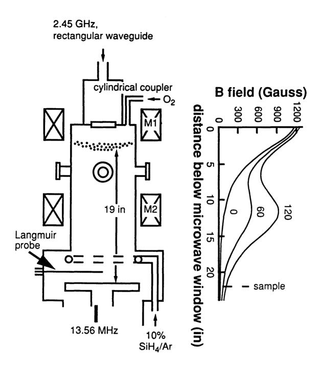
Figure 2. Schematic of ECR PECVD system with a mirror source configuration. The axial magnetic field corresponding to 170 Amps in M1 and varying the current in M2 from 0 to 60 to 120 Amps is included.
