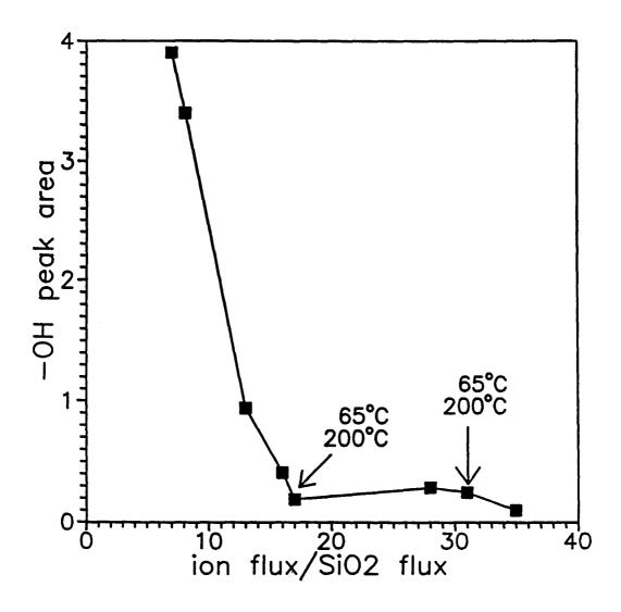
Figure 9. Decrease in the relative -OH peak area, measured on FTIR spectra, as the flux ratio is increased. Where temperature is indicated, the temperature was fixed. All other data are for a floating temperature of  $120^{\circ}$ C.
