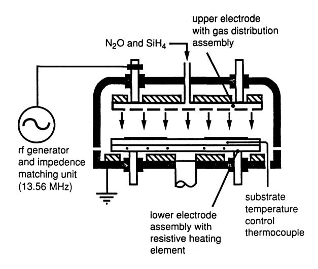
Figure 1. Schematic of rf PECVD system, from A. Kiermasz, A.A. Chambers, A. McQuarrie and M. Stephens, Semicon East, September 1986, Boston, MA.
