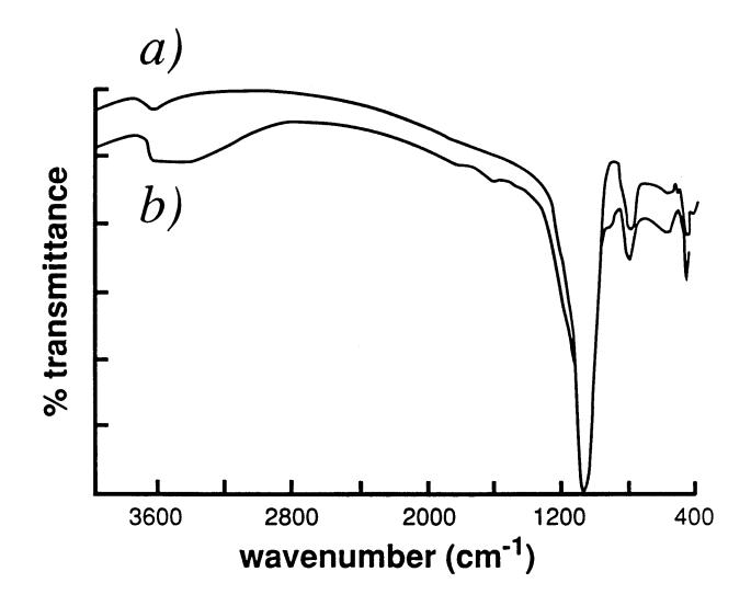
Figure 4. Fourier Transform Infrared Spectra of a) an ECR oxide grown with N<sub>2</sub>O and 10% SiH<sub>4</sub> in N<sub>2</sub> with temperature floating up to 120°C and b) an rf PECVD oxide grown with N<sub>2</sub>O and 2% SiH<sub>4</sub> in N<sub>2</sub> with temperature fixed at 200°C.
