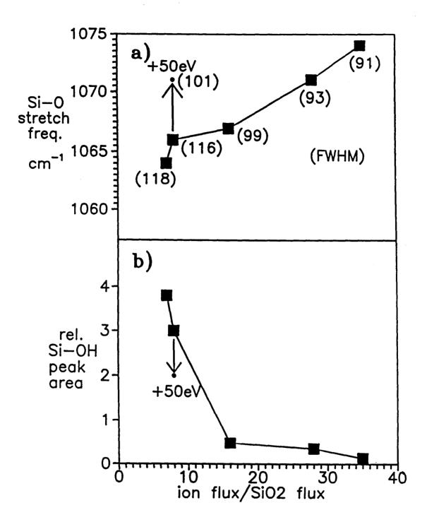
Figure 7. Changes, as the flux ratio is increased, in a) the Si-O stretching frequency and its full-width-at-half-maximum (shown in parentheses), and b) relative Si-OH peak area. Included are changes that occur by increasing the mean ion energy to 50 eV by using rf bias during deposition.
