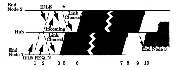
Figure 6 The Operation of Demand Priority on a Single Hub
