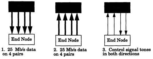
Figure 2 The Link Protocol States in Half Duplex Operation
