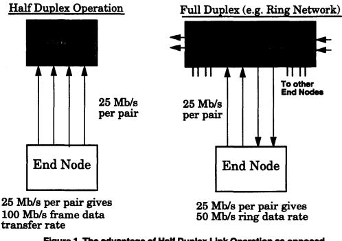
Figure 1 The advantage of Half Duplex Link Operation as opposed to Full Duplex Link Operation. Assumes 25 Mb/s transmission on each Category 3 cable physical layer.
