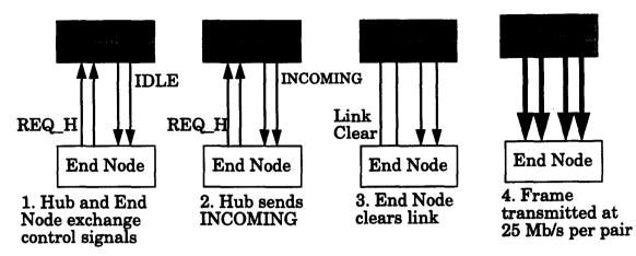
Figure 5 Link Protocol Sequence of the End Node receiving a Frame
