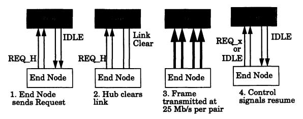
Figure 4 Link Protocol Sequence of the End Node transmitting a Frame
