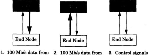
1. 100 Mb/s data from2. 100 Mb/s data from3. Control signalsHub to End NodeEnd Node to Hubin both directions
