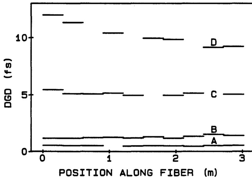
Fig. 2. Differential group delay DGD versus position along the fiber for four fibers of various core ovalities. Line segments indicate relative positions of the fiber sections; broken fibers resulted in some missing segments. A: Corning SMF-28, unknown ovality. Experimental fibers; B: 0.012 ovality; C: 0.093 ovality; D: 0.157 ovality.
