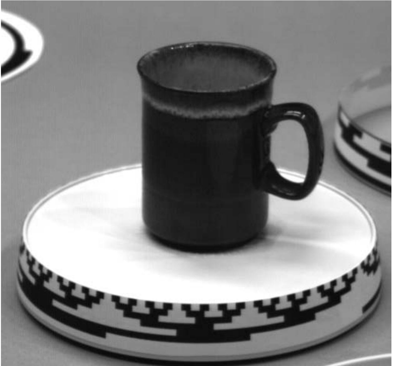
Figure 5: Input image of object (cup), turntable, and position coding ring
