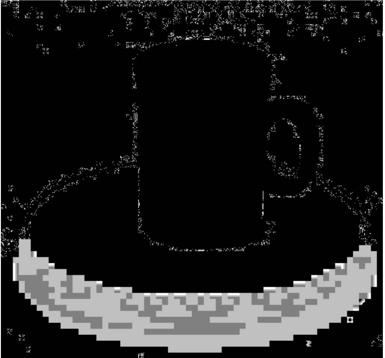
Figure 6: Thresholded image: black binary code = dark gray, white binary code = light gray, background = white, object = black.
