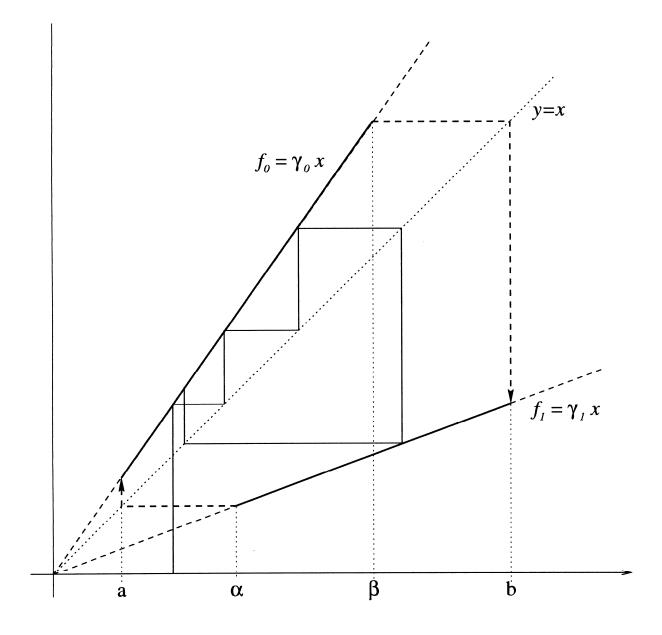
Figure 2: An example of a piecewise linear map with hysteresis and a typical trajectory
