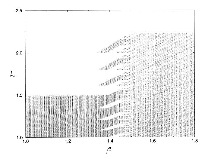
Figure 1: Graph of the global attractor of a piecewise linear map with hysteresis. The global attractor L is plotted as function of the parameter  $\beta$ .
