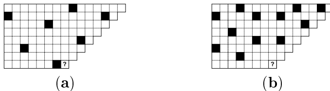
Figure 9: Pixels in causal neighborhoods indicating d_{ij} was probably: a) large. b) small.
