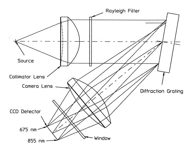
The lenses are formed by molding. F2 glass was chosen, in combination with an invar support structure, to improve stability of image position and focus with temperature changes.
