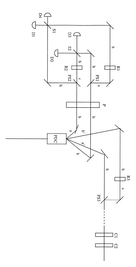
the active cells C1 and C2. letters h, v and P the polarization rotator used by the Preparer, D1-D4 detectors and C1,C2 active optical elements. The dotted line represents a long optical path, and the Fig. 1. PDC represents a parametric-down-conversion-cristal, S1,S2 regular beamsplitters, PS1-PS3 polarizing beam splitters, R 90 polarization rotators, denote polarization directions. The signal from the detectors is proccessed by electronics (not illustrated in the picture) which then controls
