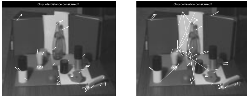
Figure 1: LEFT: The SVD method applied with \mathbf{G} as in Eqn. (1) leaves out many points due to ambiguities cause by rogue points. RIGHT: The SVD method applied with just point correlation yield non-sense results.
