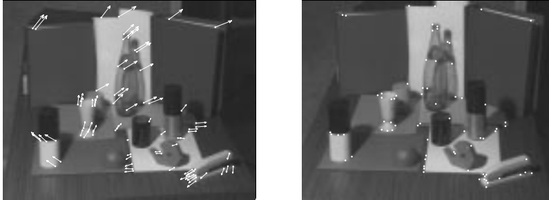
Figure 2: SVD matching with correspondence strength as in Eqn. (2). Disparities are overlaid onto the left image and matching corners onto the right one. Notice how the method managed to find the correct correspondences in difficult areas such as in the back of the stapler. (Images courtesy of INRIA)
