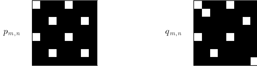
Fig. 4. Two possible halftone dot patterns for a constant gray patch at the graylevel g = 0.125 . This example leads to the conclusion that FWMSE can favor a less visually preferred pattern, i.e., \mathcal{W}(x, p) > \mathcal{W}(x, q) .
