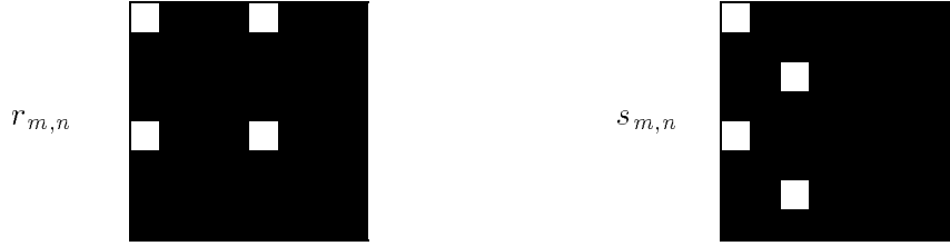
Fig. 5. Two 8 by 8 halftone renditions, r_{m,n} and s_{m,n} , of a constant gray patch of graylevel g = 1/16 . Using a modified Mannos-Sakrison visual model at 300 dpi and 12 inches viewing distance, we have 0.6911 = \mathcal{W}(x, r) > \mathcal{W}(x, s) = 0.6764 , illustrating a less visually pleasing pattern can incur a smaller frequency weighted mean squared error.
