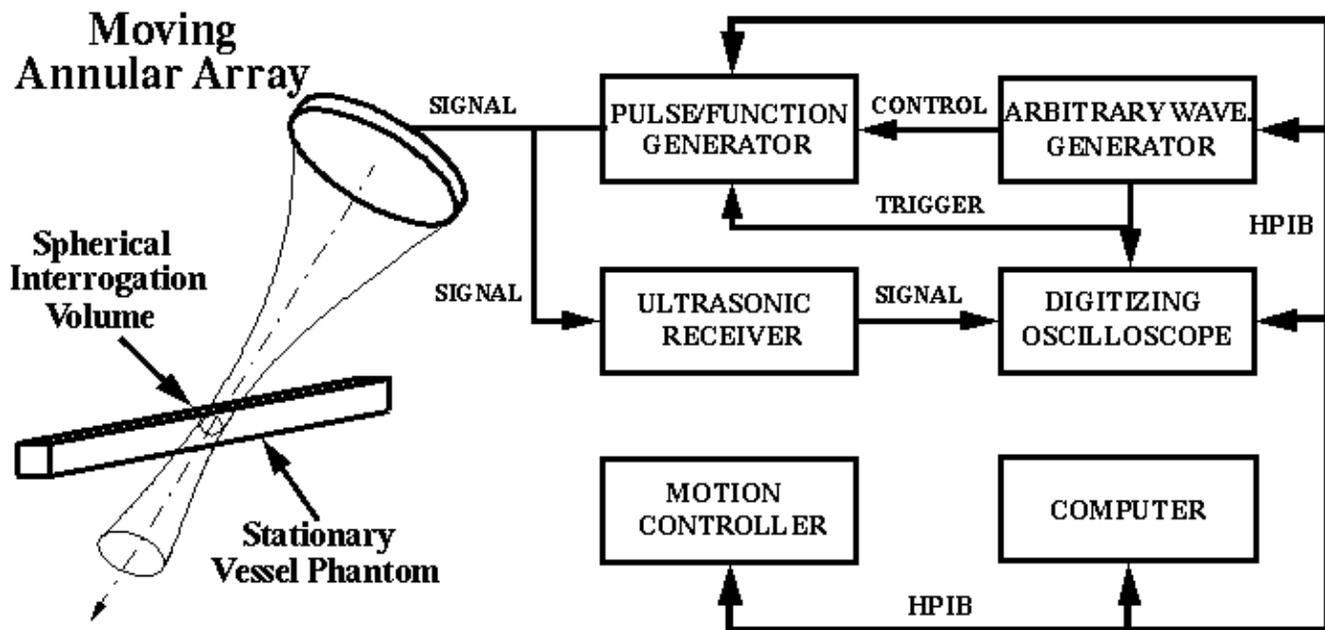
**Figure 2: System for measuring real flow.**
