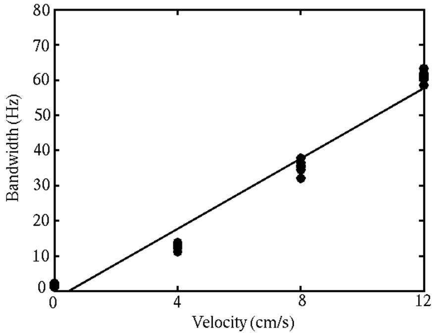
**Figure 6: Bandwidth versus velocity for real flow. Transducer angle = 75°; two-way pulse length = 0.6 mm.**
