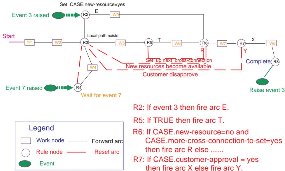
Figure 3: SOMET path provisioning OpenPM process
