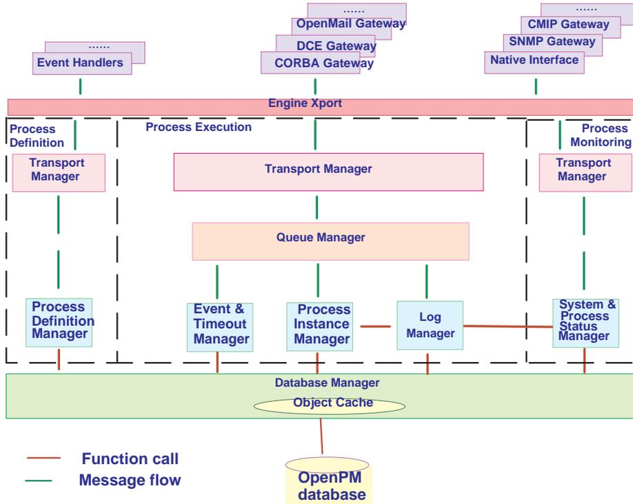
Figure 2: OpenPM component structure
