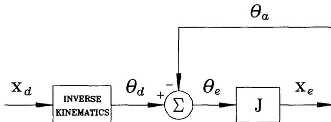
Figure 2: Modified Section of the Hybrid Control Scheme
