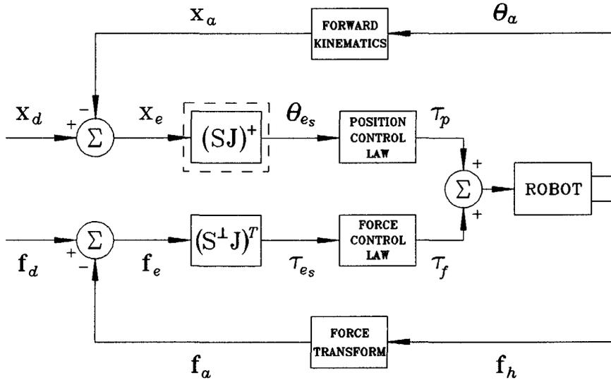
Figure 4: A Stable Hybrid Control Scheme
