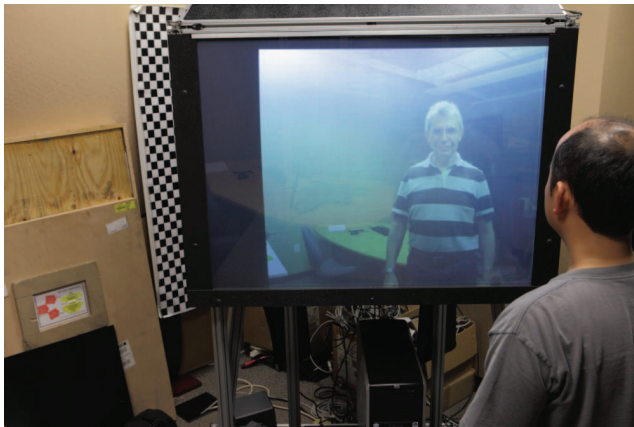
Fig. 6. Enabling eye contact. As the local user moves from the left side of the display to the right, the image of the remote user is automatically shifted so that the camera, local user's face, and remote user's face is always collinear. This way when the local user looks at the face of the remote user, he/she is always also looking into the camera, which captures the 'eye contact' view. The black bars in the screen in the top and bottom images serve to indicate the limits of the shared area between the two users. This subtly encourages local and remote users to position themselves such that the shared area is as large as possible, as is the case in the middle image.
