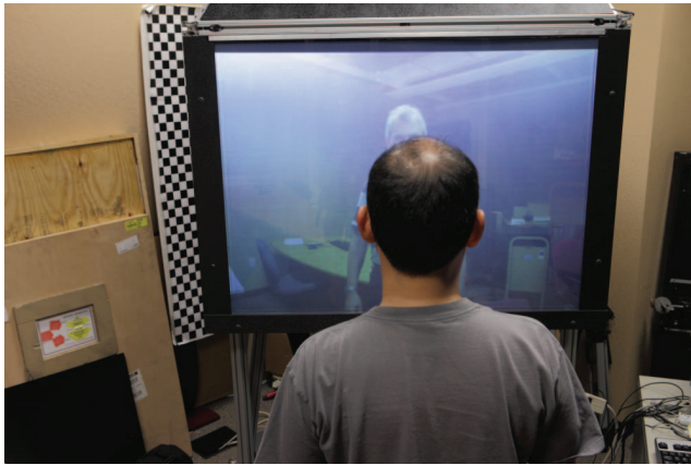
Fig. 7. Ensuring gaze awareness. As the remote user's image is shifted, the shared media (shown here digital composited) layer is also shifted correspondingly to ensure a correct rendering of the remote user's gaze direction with respect to shared content. At the same time, the users can make eye contact if they look at each other in the eye.
