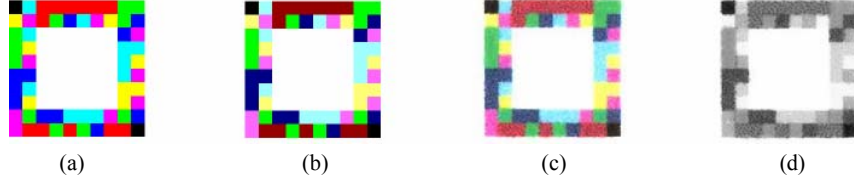
Figure 4: Example color tile deterrent with 64 tiles (enlarged for legibility). The upper left and lower right corners each contain four non-payload indicia tiles used as part of the authentication algorithm. The remaining 56 tiles store the payload. (a) Digital with no compensation, (b) Digital with GPC, (c) Color scan of the printed GPC digital, and (d) Grayscale scan of the printed GPC digital.
