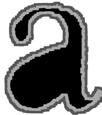
Figure 5. Character “a” with salient perimeter search areas indicated: porosities in the lightest (middle) zone, just interior to the glyph perimeter; and satellites in the outermost zone, just exterior to the glyph perimeter.
