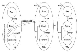
Fig. 6. State diagram of Load Balancer
