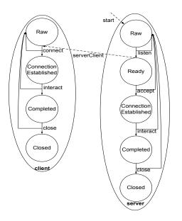
Fig. 4. State diagram of Client-Server handling failure
