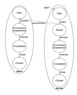
Fig. 1. State diagram of Client-Server
