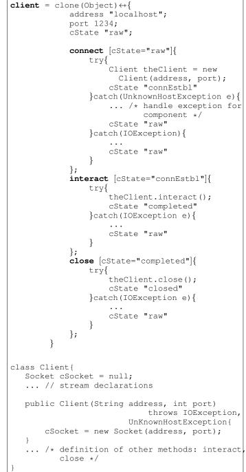
**Fig. 5:** Client-Server example: Client—Handling component failure in the object and not in the component
