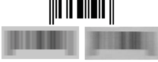
Fig. 1. An original, digital barcode (top), a simulated printed + imaged version generated using the linear model in (2) (left), and an actual printed + imaged version of the same barcode, captured in motion (right). Though noise has been ignored, the model reasonably represents the actual image.
