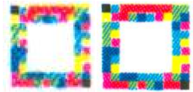
Figure 5. LJ printer + 8200 scanner at 5x5 and 10x10 pixel (at 600 dpi) size (left, right).
