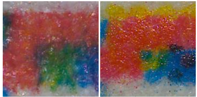
Figure 7. Up-close 5x5 pixel size (at 600 dpi original image printing specifications) captured using the Dr. CID imager showing the ink wicking (IJ printing, left) and the color plane mis-registration (LJ printing, right).
