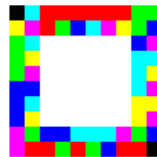
Figure 2. 3D barcode “color tile” configuration used for the test sheets. The individual tiles, of which there are 64 in total, sized 5-10 pixels on a side at 600 dpi.
