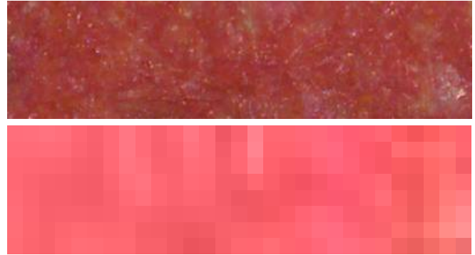
Figure 9. Representative swatches of red color tiles (images shown extend across three red color tile modules atop left images of Figures 3 and 4), for Dr. CID (upper) and 8200 scanner (lower). While the two images represent the same physical area, the Dr. CID image was captured at 12X the resolution in both the x- and y-direction. The Dr. CID image shows evidence of (much) higher substrate variability and less saturation (comcomitant with lower contrast overall); however, it does not show drastically higher hue variability.
