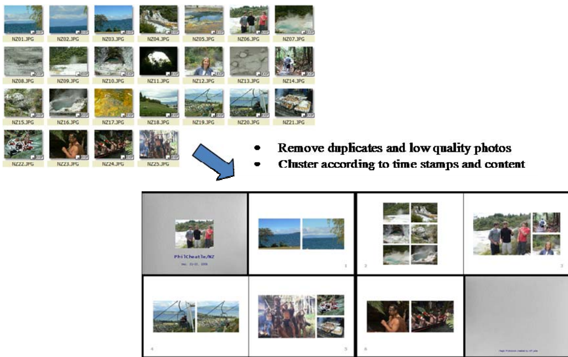
Figure 4: Using photo analysis to automatically create a photobook from a set of photos.
