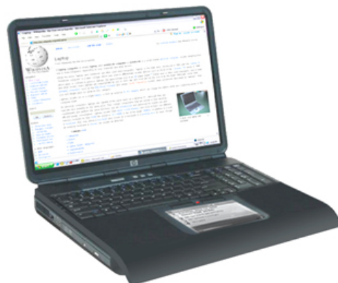
Figure 10. Papyrus prototype placed on a conventional notebook to give the papyrus form factor
