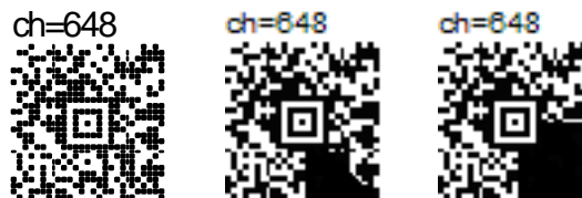
Fig. 1. Example of original and damaged Aztec Code 2D barcodes (ch=648 indicates maximum bits to use for encoding characters). Original size was 20 x 20 mils per module. Payload is 456 out of 648 payload bits (30% ECPSA). Images show no damage (left), 12.5% damage (center) and 25% damage (right).
