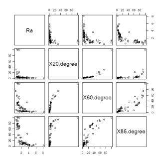
Fig. 1. Scatterplot of surface roughness, Ra in microns, and 20°, 6°0 and 8°5 gloss measurements in gloss units.
