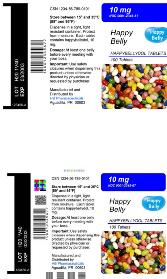
Figure 1. Label template (top) and label template with variable copy holes filled with explicit security and point of sale marks (bottom).
