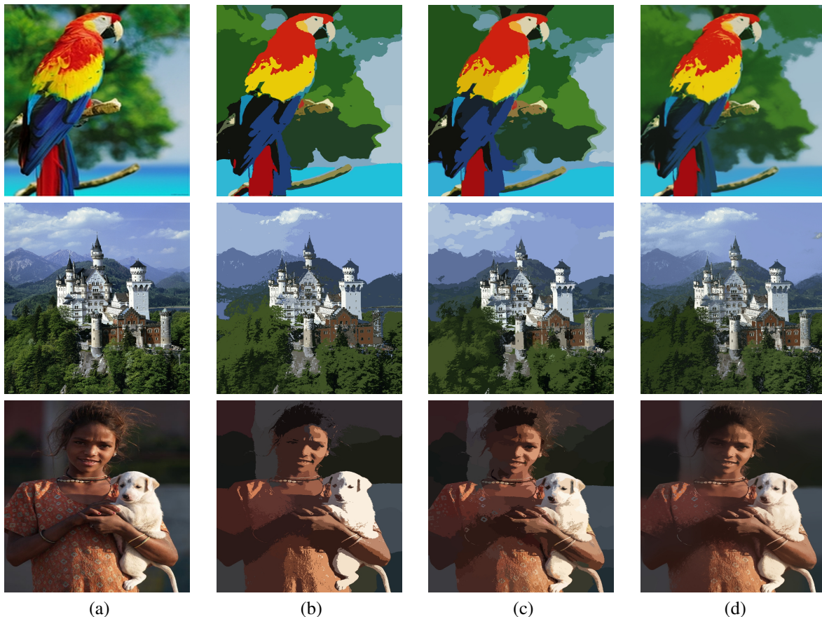
Figure 1. Image segmentation example: (a) the original image (b) the result of standard Mean Shift segmentation (c) the result of fast Mean Shift segmentation (d) the soft segmentation variant of the fast Mean Shift. Note similar hard segmentation results in (b) and (c); the proposed method is more than 1000 times faster than the original Mean Shift.
