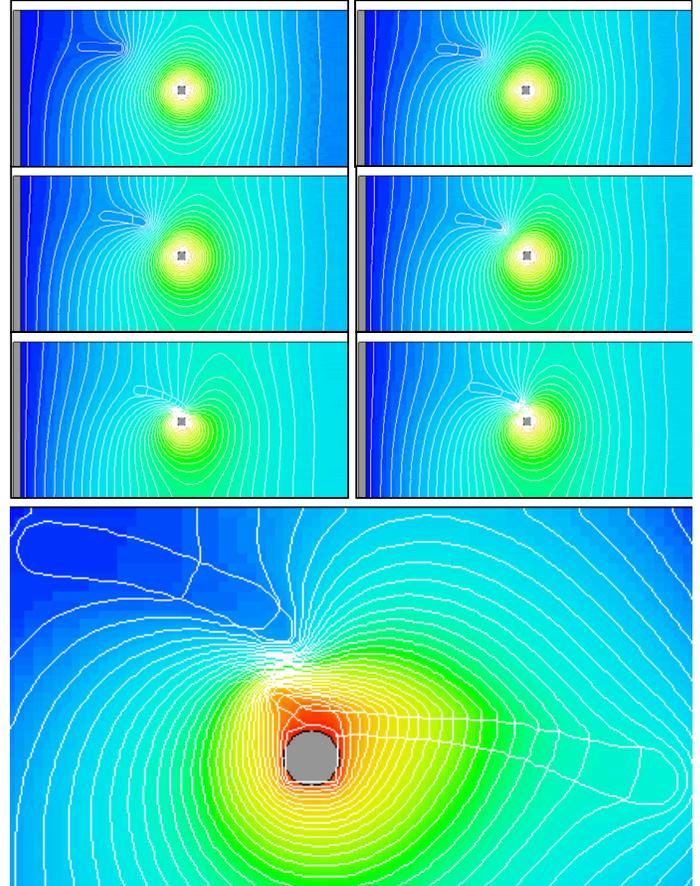
**Fig. 3.** Simulation of dielectrophoresis driven axon migration. The set of images at top shows a transient simulation of single axon migration under an electric field generated by a pin electrode. The image at bottom is a snapshot of a simulation where two axons are fused by dielectrophoresis using a pin electrode. Axons are outlined in white. Also shown are the iso-potential curves.
