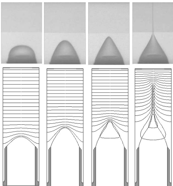
**Fig. 4.** Transient sequence of the Taylor cone formation: simulation and experiment comparison. Experimental images are shown at the top row. Simulation results are shown at the bottom row. Their correspondence is indicated by the vertical alignment. The experimental images courtesy Dr. D. Sobek of Agilent Technologies Inc.
