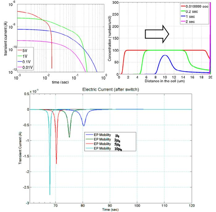
**Fig. 6.** Simulation of charge screening effect using a parallel-plate cell. Top-left image shows the electric current as function of time and driving voltage, top-right image shows the evolution of the species concentration as function of time and space, the bottom image shows the electric current readout after switching the applied voltage.
