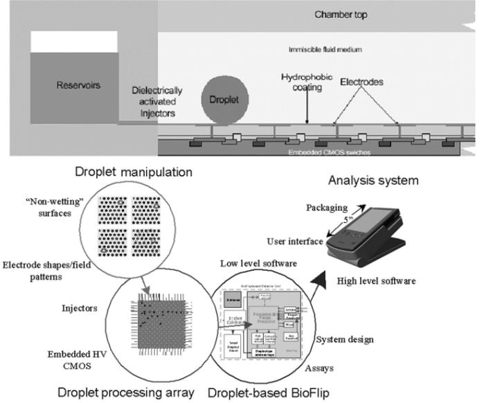
**Fig. 1.** Example droplet-based digital microfluidics architecture. Above is an elevation view showing the layered structure of the chip. Below is a diagram illustrating the system. Courtesy professor Peter Gascoyne, M. D. Anderson Cancer Center.
