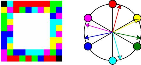
**Figure 1. Color tile deterrent (left) and spectral pre-compensation colors (triangles) printed to obtain intended colors (circles) after printing and scanning.**
