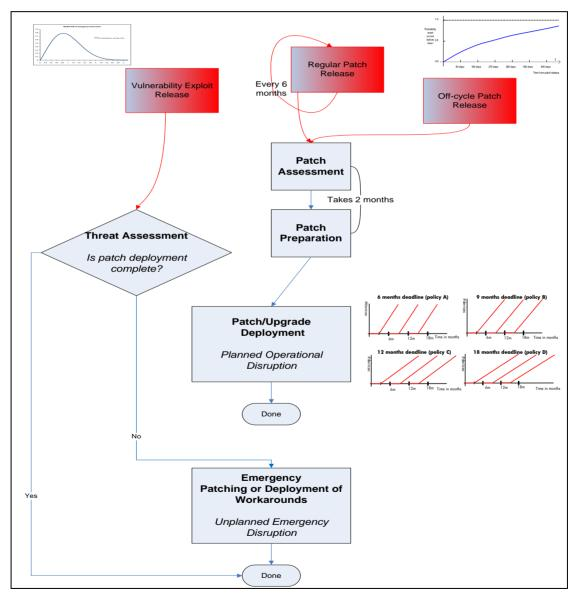
Figure 1. Activity diagram of a typical patch management process.
