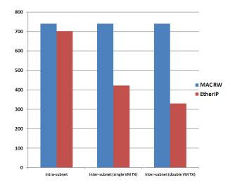
Figure 9: Inter-subnet Throughput Results in Mbps.
