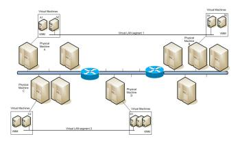
Figure 1: Virtual to Physical network mapping.
