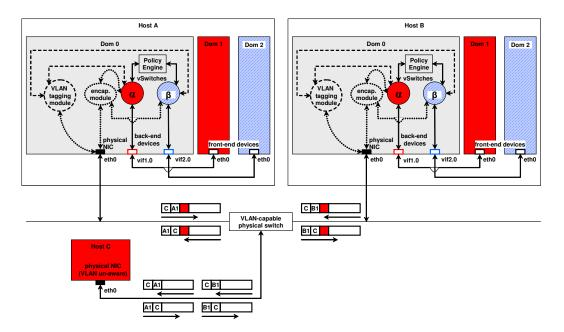
Figure 7: Prototype implementation of VLANs as security domains.
