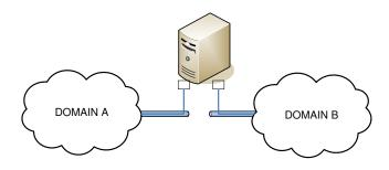
Figure 3: An example dual-homed host with two NICs for inter-domain flow control between two security domains.
