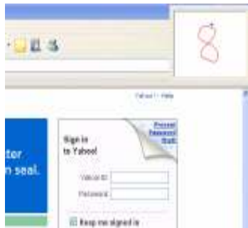
Figure 1. Application login using a doodle. Visual feedback while doodling is provided using a small window.
