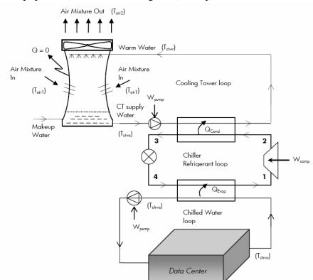
Figure 3: Data Center Facility Cooling infrastructure
