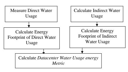
Figure 8: Flowchart for calculation of data center water usage energy metric.
