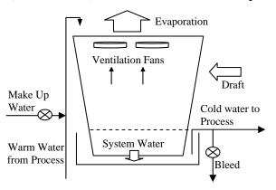
Figure 4: Cooling tower schematic
