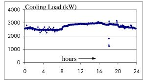
Figure 5: Typical demand profile in an IT facility
