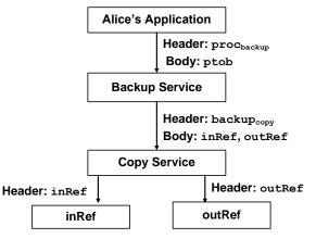
Figure 7. Permission flow in sample use case showing the certificates used for invocation and delegation and where they appear in the SOAP message.
