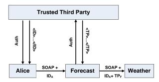
Figure 2. Use of the Transited Provider SAML profile.
