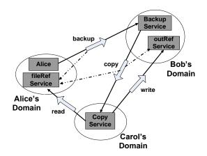
Figure 3: Illustration of the sample use case. Heavy arrows denote service invocation. Dotted lines, service delegations. For example, Alice invokes the backup service delegating to that service the right to use the fileRef service. Bob's backup method's invocation of this service is
