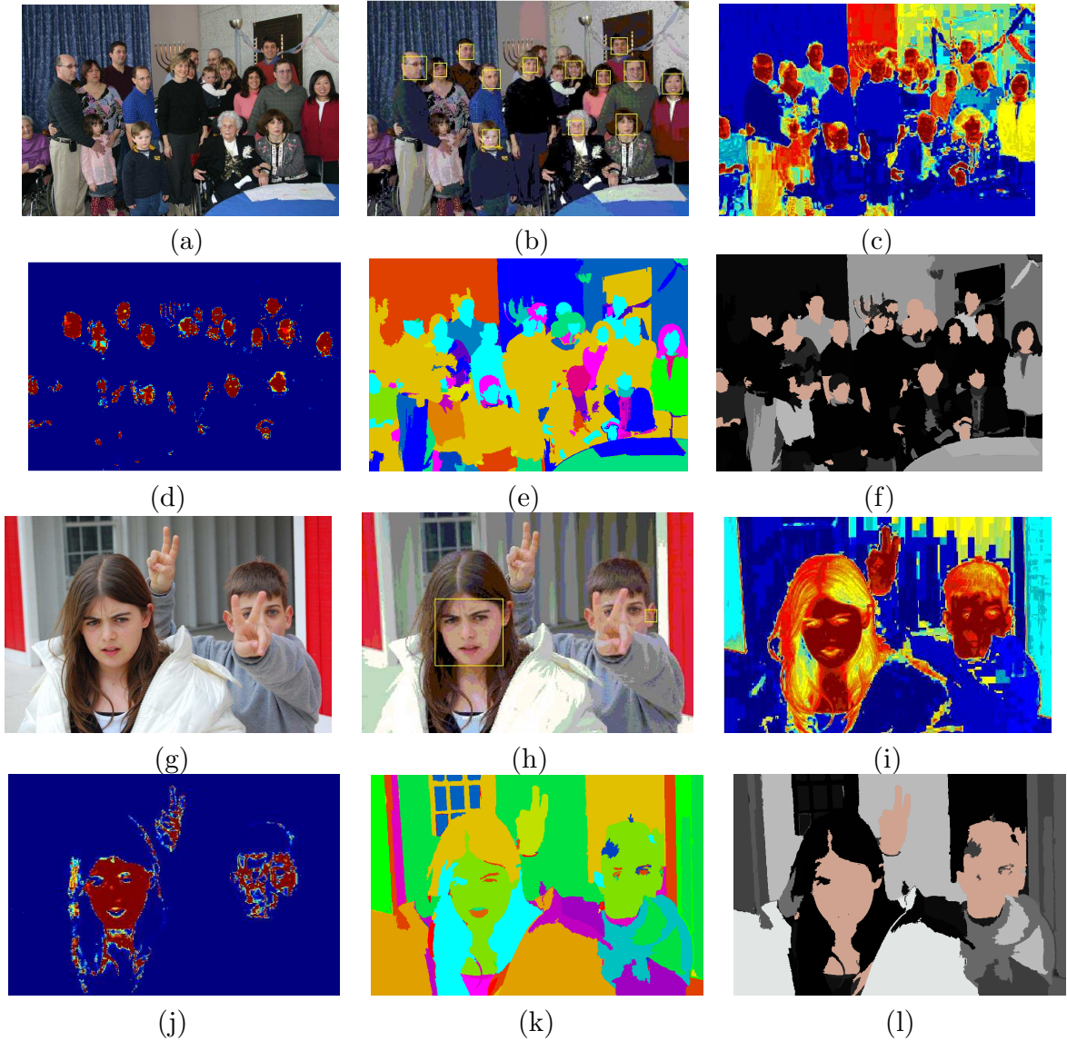
Figure 4: Examples of skin detection and tagging for two images (a) and (g). Face detection results are shown in (b) and (h), respectively. (c) and (i) show the corresponding global skin maps. Face detection and the global skin map are used by the per-face learning algorithm to compute a per-face skin model. This model is applied to the rest of the image to find the improved skin maps in (d) and (j). Segmentation for each image is shown in (e) and (k). Finally, (f) and (l) depict the skin tagging for each segment.
