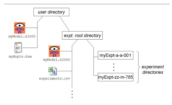
Figure 21: Diagram of the directory structure for a single experiment set
