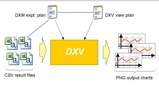
Figure 23: Block diagram describing input dependencies and outputs for DXV
