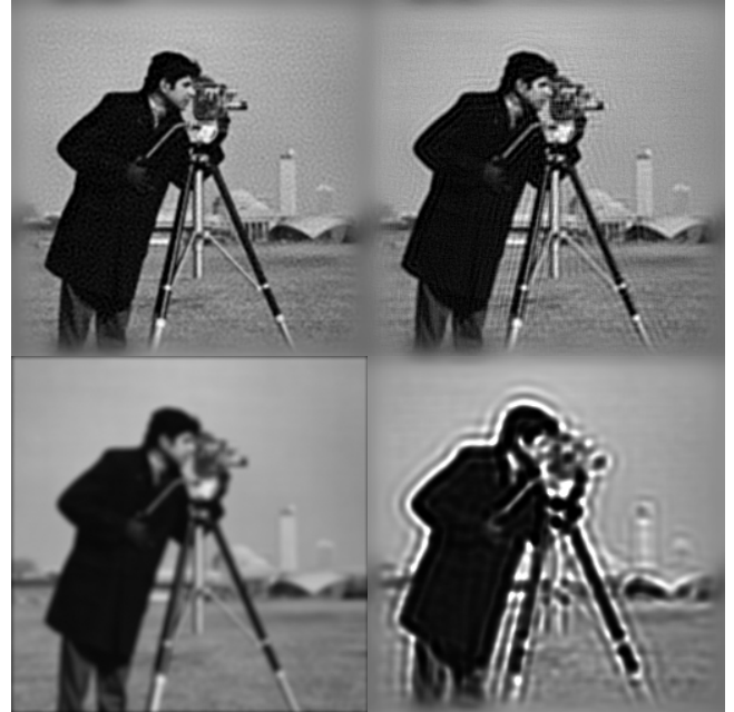
Figure 6: (Top left) Our deblur method, (Top right) Wiener method, (Bottom left) Long exposure image, and (Bottom right) blind deconvolution (deconvblind) in MATLAB
