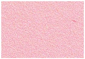
Figure 5: Flocculation during curing, 200x magnification. No polarisers.
