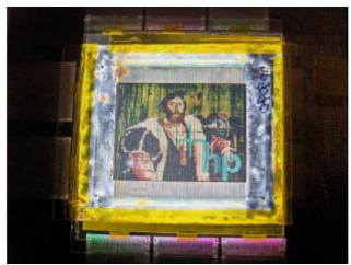
Figure 1: Picture of bistable, plastic, full colour prototype
