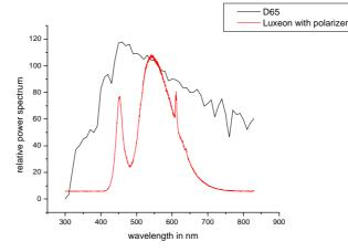
Figure 3: D65 spectrum and spectrum of a Luxeon backlight in combination with a polarizer.
