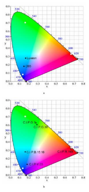
Figure 4:The white dots represent the chromaticity coordinates of the NTSC standard. a) chromaticity shift caused by different spectra of light source. b) chromaticity coordinates for different pigments calculated with the spectrum of the LED Luxeon instead of a D65 spectrum.
