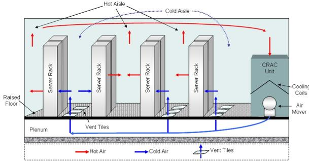
**Figure 1. Typical Raised Floor Data Center Configuration**
