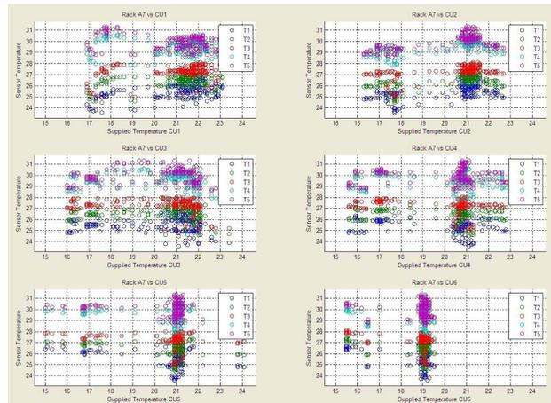
**Figure 9. Crac Units Supply Temperatures Vs. Sensor Temperatures (Experiment A)**
