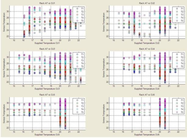
**Figure 10. Crac Units Supply Temperatures Vs. Sensor Temperatures (Experiment B)**
