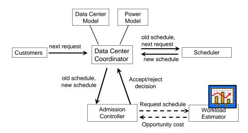
Figure 1. Data center coordinator. Architecture showing communication internal to data center coordinator and outward to customers.
