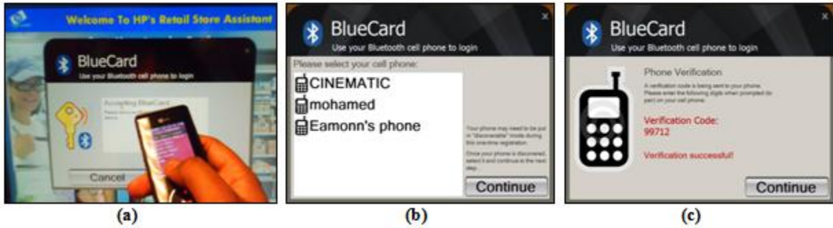
Figure 5: Screen-shots of BlueCard: (a) Login using BlueCard on device. (b) Device discovery during registration. (c) Challenge-response verification during registration.
