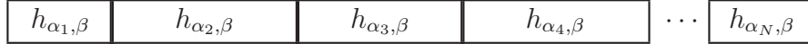
Figure 6: Arrays with sequence of filter coefficients that are pre-computed for image resizing, and repeatedly used in the vertical (or horizontal) resampling computations.
