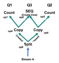
Figure 11: The progressive, bottom-up operator scheduling inside a query plan (from Fig.9b).
