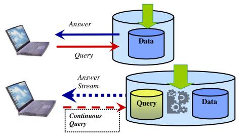
**Figure 1:** DBMS are characterized by requests followed by synchronous responses. In DSMS a continuous query is registered once and the responses are received as a stream asynchronously.
