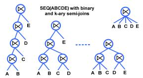
Figure 7: Different options to implement long event sequences (e.g. A, B, C, D, E) using binary and/or multi-way semi-joins.
