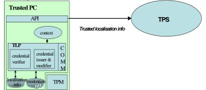
**Fig. 4.** Trusted Localisation Provider (TLP)
